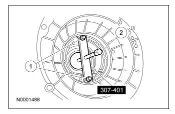
43. **NOTE:** Align the disc holes on special tool with the slot in gauge bar for correct measurement.
